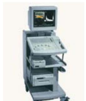
that looks much like a computer or television monitor. The image is created based on the amplitude (strength), frequency and time it takes for the sound signal to return from the patient to the transducer and the type of body structure the sound travels through.
